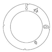
The corresponding burner marked on the index is listed above each knob on the front panel
